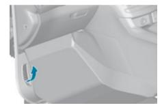
Pull the release lever. located at the bottom of the door aperture, towards you.
