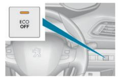
In the event of a fault with the system, this warning lamp comes on continuously. Have it checked by a PEUGEOT dealer or a qualified workshop.
