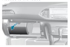
Unclip the cover by pulling at top left, then right.
