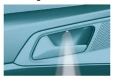
At night, the illumination of the interior opening controls on the front doors comes on automatically when the sidelamps are switched on.
