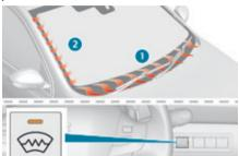
In area 1, the heating frees the wiper blades when they are stuck by snow or ice.
