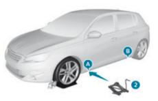
Position the foot of the jack on the ground, ensuring that it is directly below the vehicle's jacking point **A** or **B**, the one closest to the wheel to be changed.
