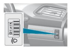
To avoid causing a nuisance to other road users, the beams of the halogen headlamps should be adjusted according to the load in the vehicle.
