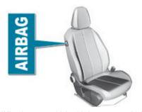
If fitted to your vehicle, this is a system which protects the driver and front passenger in the event of a serious side impact in order to limit the risk of injury to the chest, between the abdomen and head.
