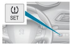
(!) SET With the ignition on and the vehicle stationary, press this button for about 3 seconds then release it, an audible signal confirms the reinitialisation.
