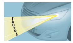
This system automatically adjusts the height of the beams from this type of headlamp, according to the load in the vehicle, to avoid causing a nuisance to other road users.
