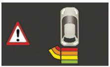
This supplements the audible signal by displaying bars in the screen or the instrument panel which move progressively nearer to the vehicle. When the obstacle is near, the "Danger" symbol is displayed.
