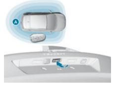
With the electronic key on your person in the recognition zone A, press the opening control then raise the tailgate.
