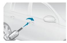
Turn the key to the front of the vehicle to unlock the vehicle, then pull the handle to open the door.
