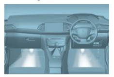
Its operation is identical to that of the courtesy lamps. The lamps comes on when one of the doors is opened.
