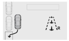
Select reverse, release the steering wheel and start moving without exceeding 4 mph (7 km/h).
