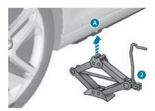
Extend the jack 2 until its head comes into contact with the jacking point A or B used, with the contact surface A or B on the vehicle correctly engaged with the central part of the head of the jack.
