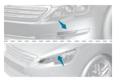
They come on automatically when the engine is started, when the lighting control stalk is in position "0" or "AUTO".
