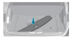
A recess in the floor well, under the boot carpet, allows the luggage cover to be stowed diagonally.
