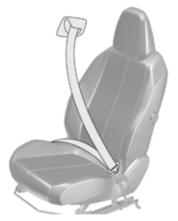
The front seat belts are fitted with a pretensioning and force limiting system. This system improves safety in the front seats in the event of a front or side impact. Depending on the severity of the impact, the pretensioning system instantly tightens the seat belts against the body of the occupants. The pretensioning seat belts are active when the ignition is on.
