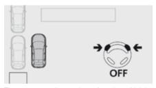
The manoeuvre is complete when the vehicle's front wheels are clear of the parking space. At the end of the manoeuvre, the indicator lamp in the instrument panel goes off, accompanied by a message and an audible signal. The assistance is deactivated: you can take
