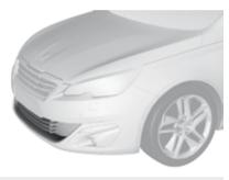
The operation of the radar, located in the front bumper, may be disturbed in certain weather conditions, for example: with accumulations of snow, ice, mud, ...
