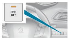
At any time, press the **"ECO OFF"** switch to deactivate the system.
