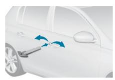
Insert the integral key in the door lock, then turn it to the rear.
