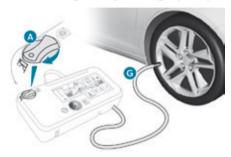
You can also use the compressor without injecting any product, to check and if necessary adjust your tyre pressures.
