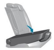
Pull the control 1 forwards, the seat backrest folds onto the cushion.
