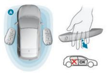
With the electronic key on your person and in the recognition zone A, pass your hand behind one of the front door handles to unlock the vehicle, then pull on the handle to open the door.
