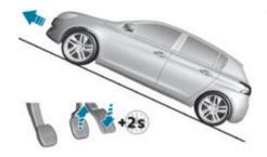
On an ascending slope, with the vehicle stationary, the vehicle is held momentarily when you release the brake pedal.
