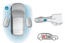
With the electronic key in the recognition zone A, press with a finger on one of the front door handles (at the markings) or press the locking control on the tailgate to lock the vehicle.
