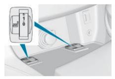
With the engine running, the front seats can be heated separately.
