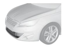
The operation of the radar, located in the front bumper, may be disturbed in certain weather conditions, for example: with accumulations of snow, ice, mud, ...
