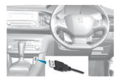
It allows the connection of a portable device, such as a digital audio player of the iPod® type or a USB memory stick.
