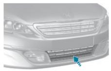
When towing, you must remove the blanking cover if your vehicle has one.
