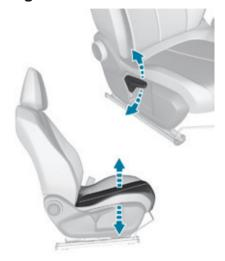
Pull the control upwards to raise or push it downwards to lower, as many times as required, to obtain the position required.
