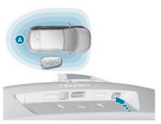
With the electronic key in the recognition zone A, press the boot locking control to lock the vehicle.
