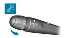
Pull the stalk to switch the lighting between dipped and main beam headlamps.
