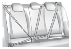
The rear seats are each fitted with a seat belt, three-point anchorages with inertia reel and force limiter (except for the centre rear seat).
